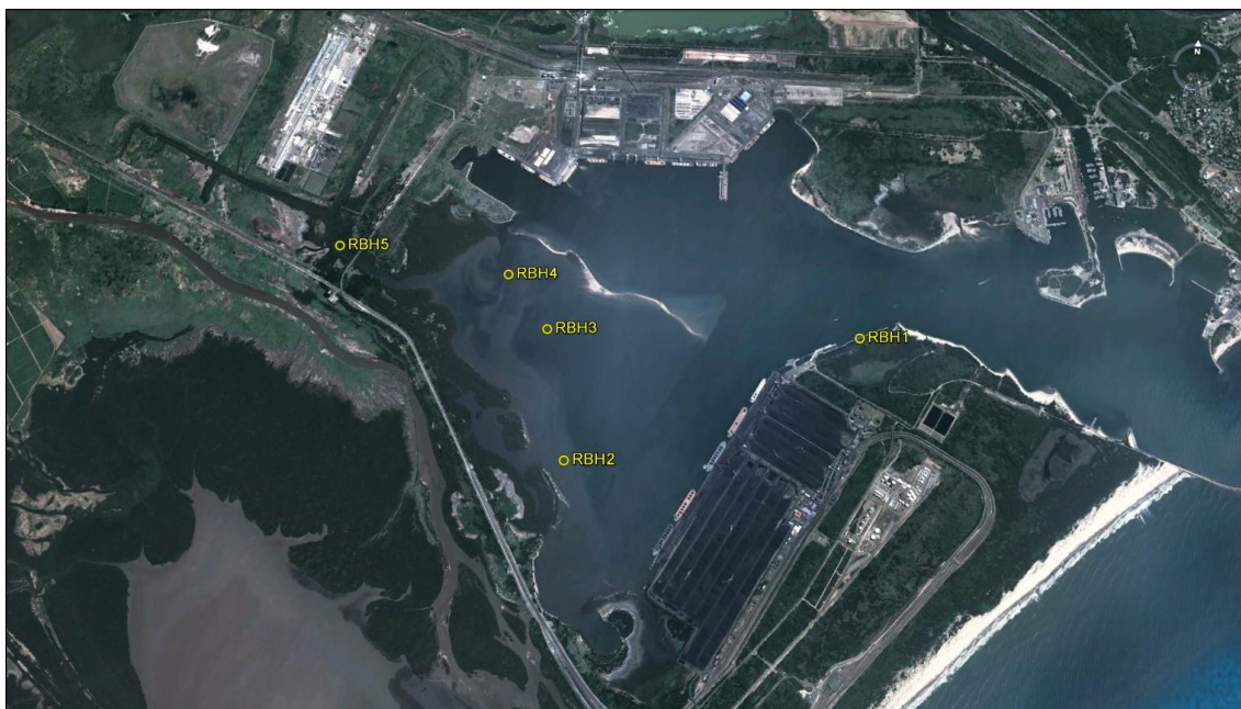
Figure 4. Aerial view of Richards Bay showing the positions of compliance monitoring stations for the Richards Bay Coal Terminal expansion dredging compliance monitoring programme. Aerial view reproduced from Google Earth.
