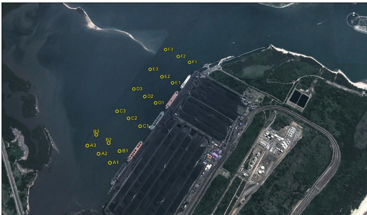
Figure 8. Aerial view of Richards Bay showing the positions where turbidity was profiled through the water column during and after dredging for the Richards Bay Coal Terminal expansion compliance monitoring programme.
