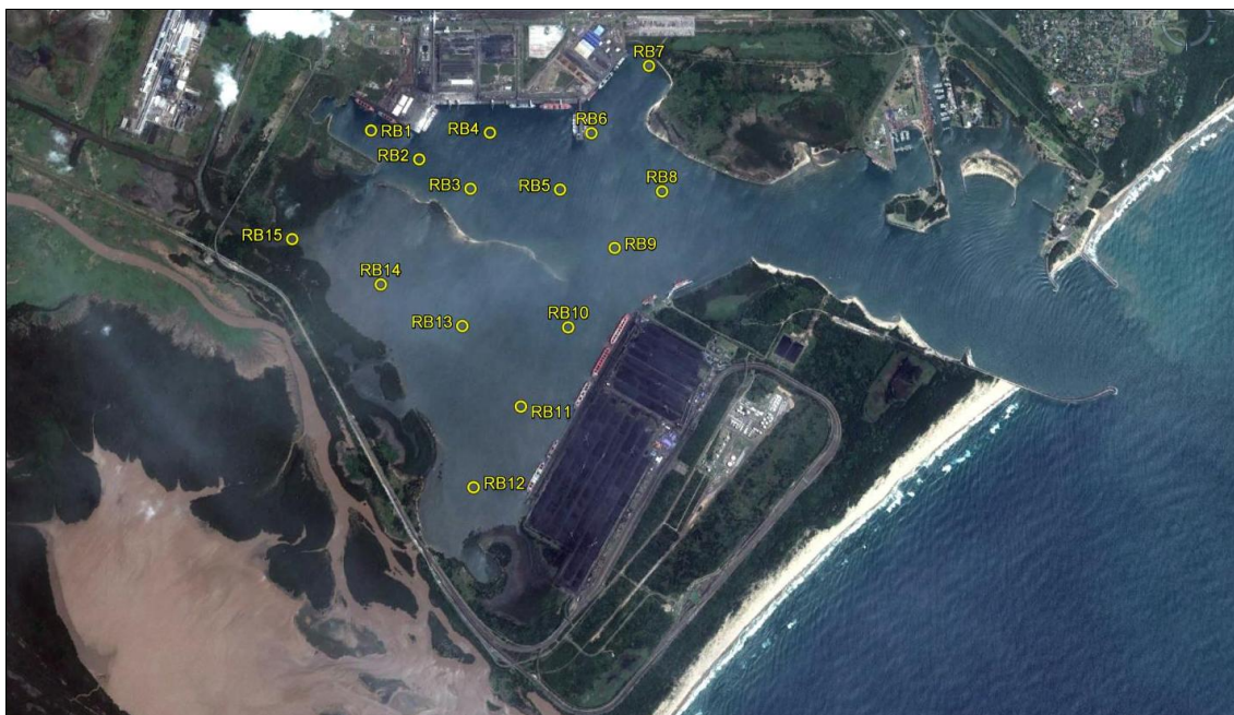
Figure 2. Aerial view of Richards Bay showing the positions where in situ water quality measurements were made and water samples were collected for turbidity and total suspended solids concentration analysis in the laboratory in February 2013. Aerial view reproduced from Google Earth.
