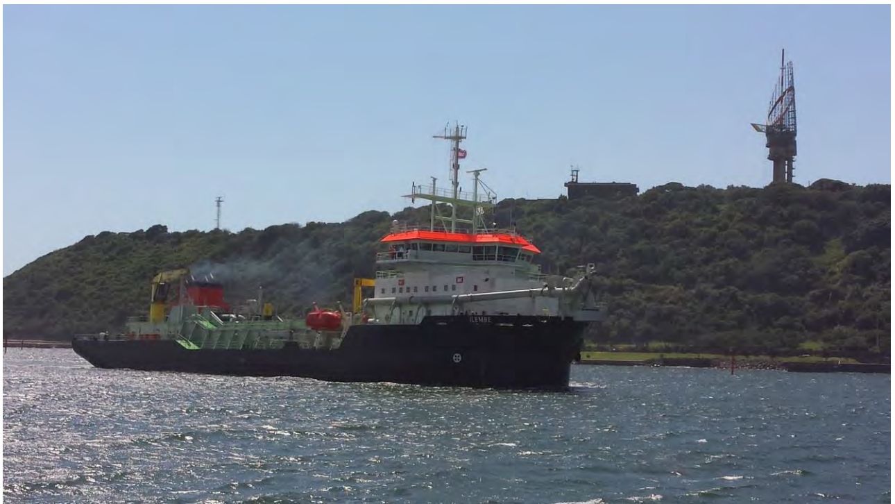
Trailer Suction Hopper Dredger (TSHD) Ilembe
