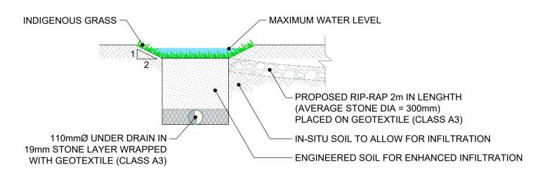
TYPICAL DETAIL OF ENHANCED SWALE WITH UNDER DRAIN (GRASSED CHANNEL) WITH OUTLET TOWARDS STREAM
