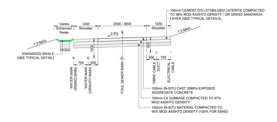
TYPICAL CROSS SECTION WITH IN-SITU CONCRETE SCALE 1:50
