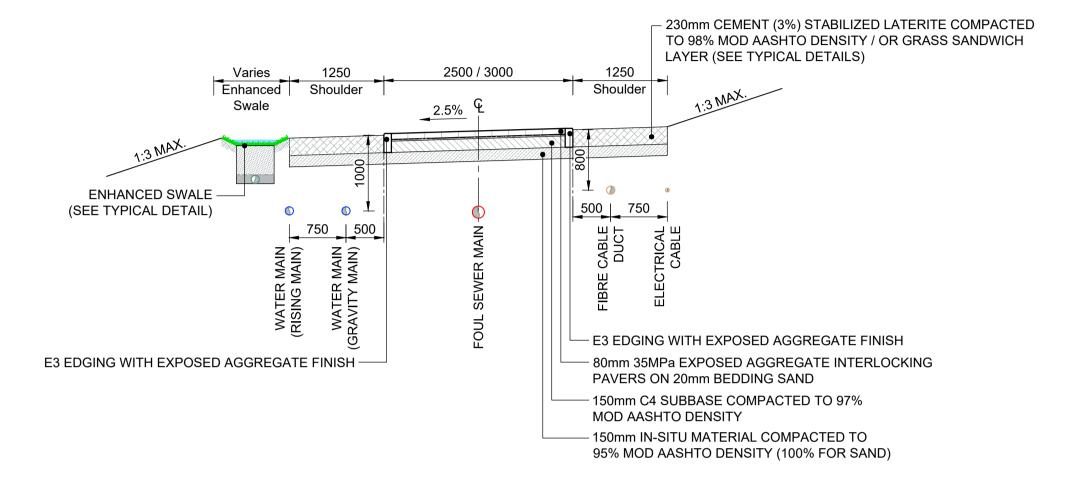
TYPICAL CROSS SECTION WITH INTERLOCKING PAVERS SCALE 1:50
