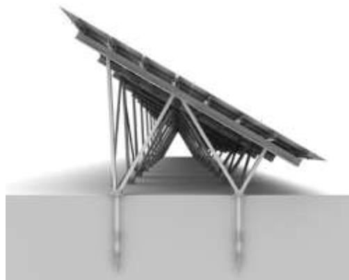
Figure 6: Rammed or screwed mounting method on fixed frame (image www.expo21xx.com )
