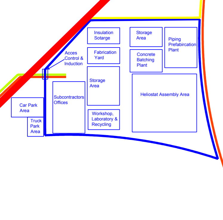
Temporary Construction Facilities Detail - Scale 1:7,000
