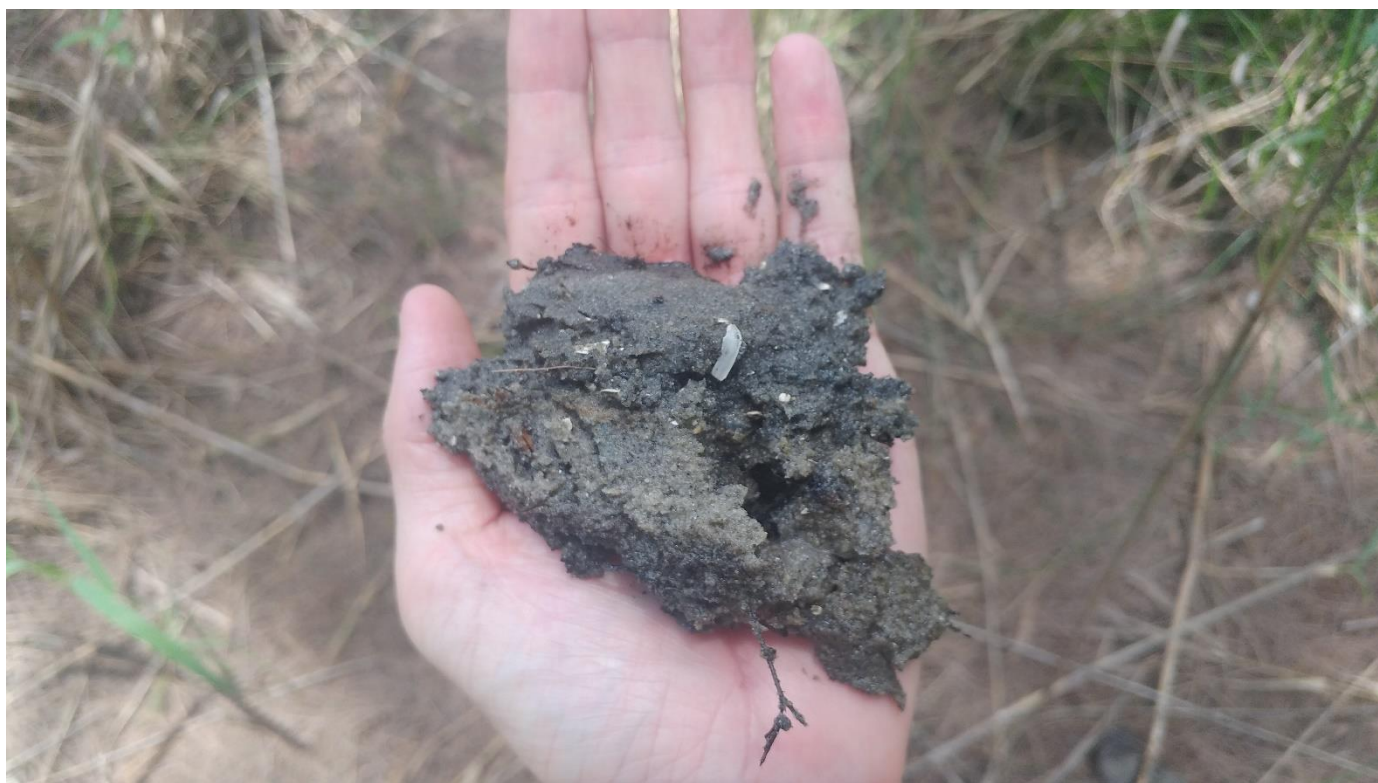
Photographs 5.5: Bleached soils drawn from soil samples taken within the bed of the artificial drainage channel showing prolonged saturation.
