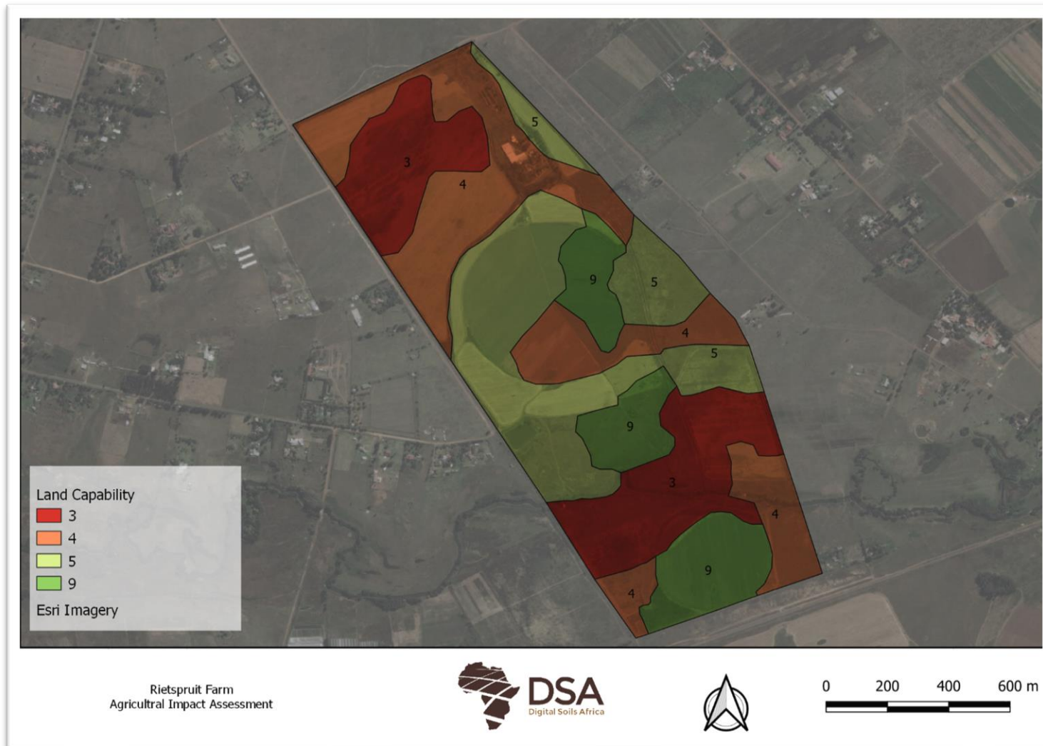
FIGURE 15: REFINED LAND CAPABILITY CLASS MAP OF THE AREA CALCULATED FROM SOIL OBSERVATIONS.
