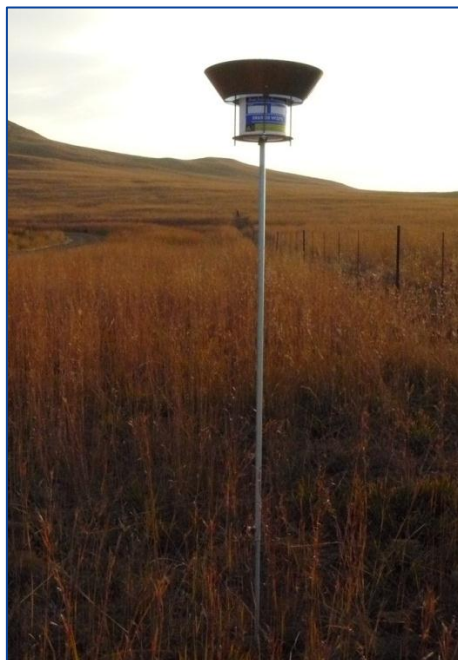
Figure 3: Photograph of dust bucket installed at location YZ DFO 04
