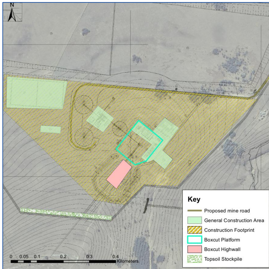
Figure 12: Site layout of the proposed Yzermyn Underground Coal Mine and related construction phase emission sources
