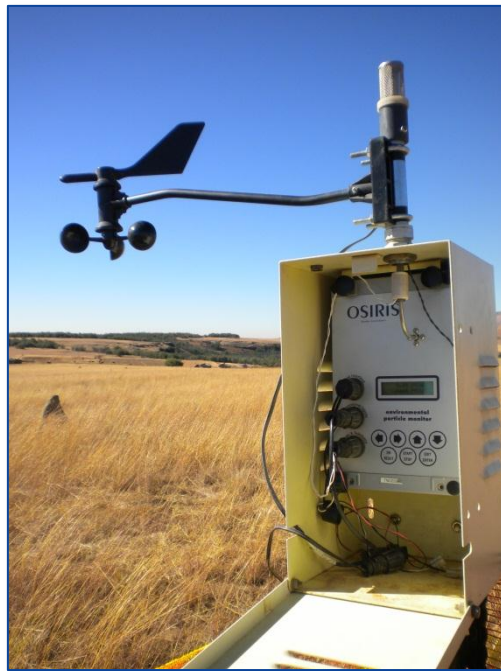
Figure 5: Osiris™ analyser installed at the proposed Yzermyn Underground Coal Mine site
