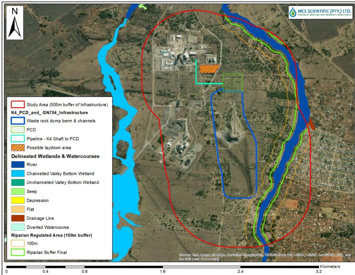
Figure 13. Proposed infrastructure footprint, 100m regulated area, and 25m aquatic impact buffer in relation to the delineated riparian habitat.
