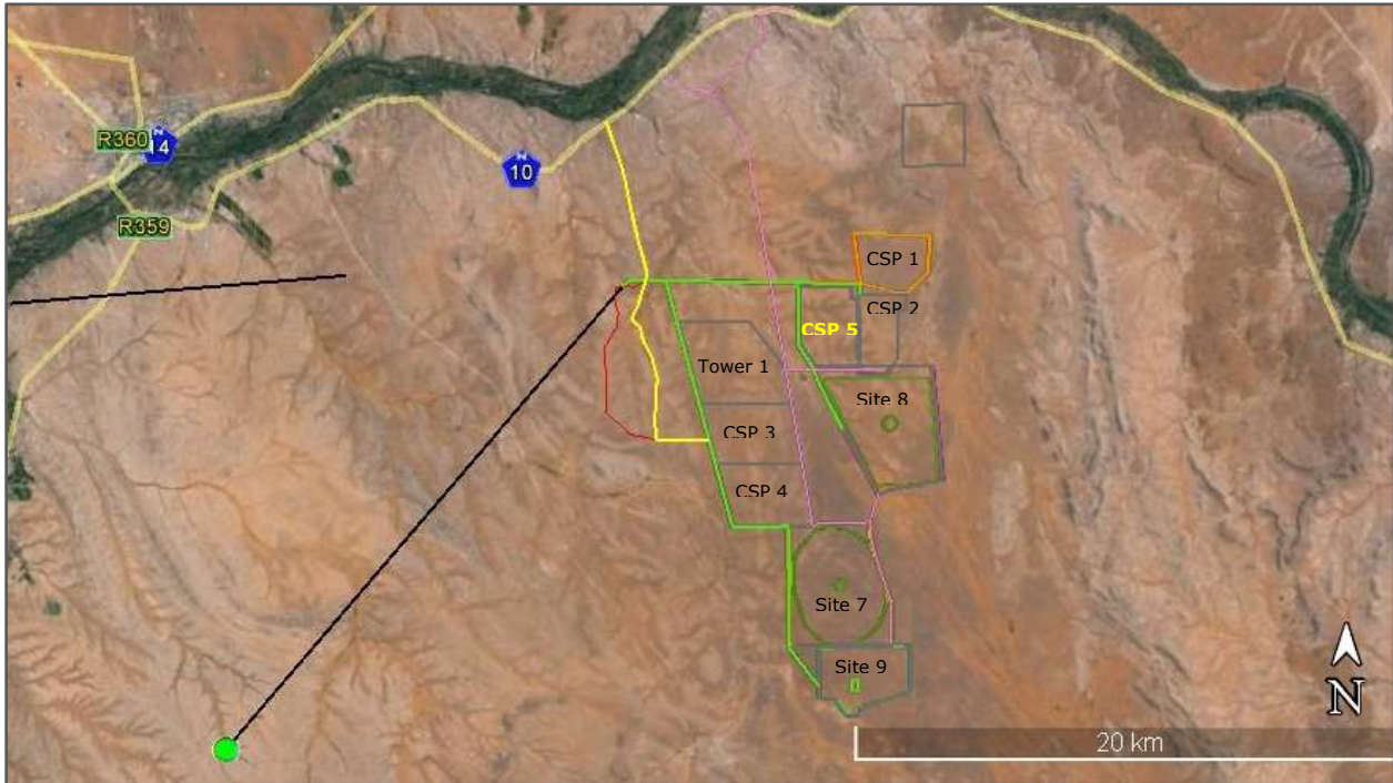
Figure 1. The proposed development area of Illanga CSP 5 within the broader Karooshoek Solar Valley Development, including all sites and infrastructure alternatives (access roads (red and yellow), pipelines (pink) and power line route (green) and the power lines (black) that will link the facility to the ESKOM grid at the proposed ESKOM MTS substations (green)).
