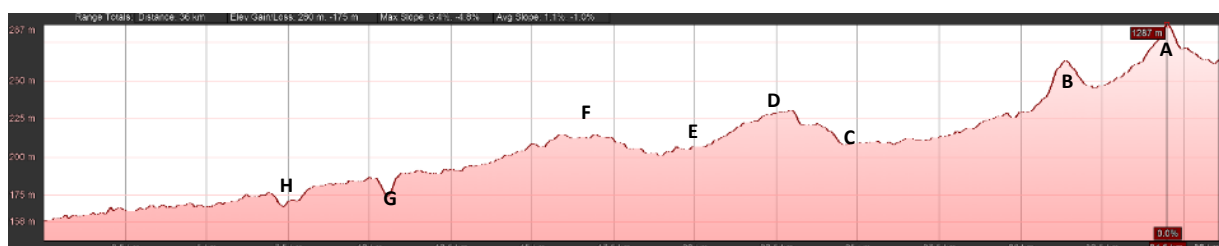
Figure 22: Elevation profile (Google) of the power line route from Emil substation to the Olifantshoek substation). Important topographical features: A = andesitic lava outcropping; B = chert hill; C = low lying calcrete plain; D & F = elevated deep regic sand; E = exposed chert area; G = Ga-Mogara River, H = Ga-Mogara River
