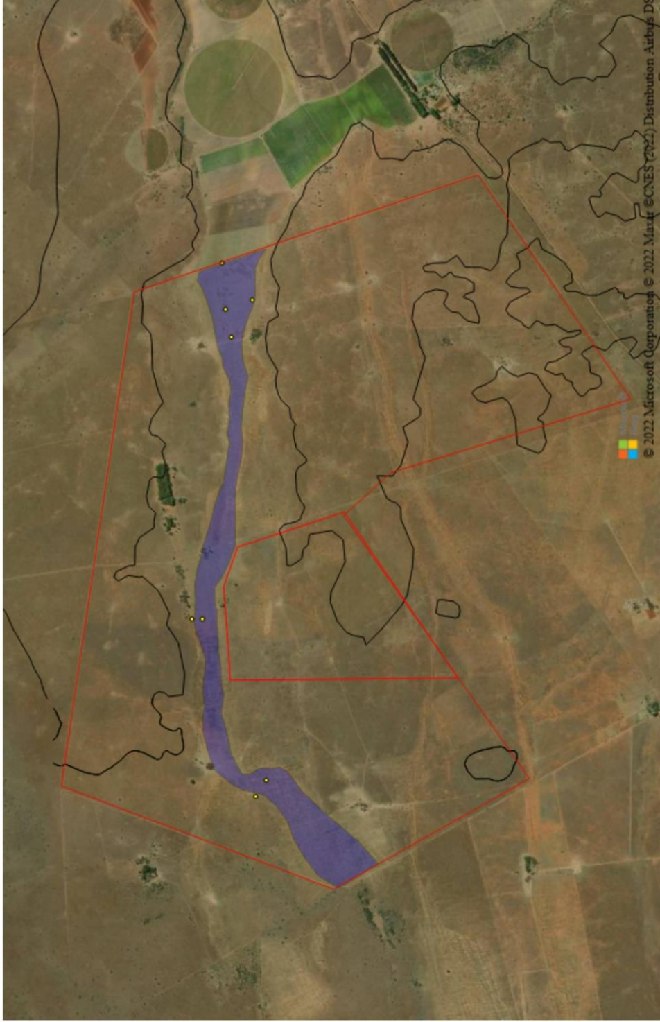
Map 3: Surface water delineation map of the proposed Kiara PV solar development (Phase 5) on the Farm Hollaagte 8 near the town of Lichtenburg. A large central drainage area occurs in the study area. The system is largely devoid of riparian and wetland conditions with a few depression wetland areas only forming toward the eastern portion of the study area. This will decrease the sensitivity of the system. However, it does still function as a surface water system and wetland areas in the eastern portion confirm a shallow groundwater table. It will also play an important role in terms of the local groundwater resources, especially so since it forms part of the Bo-Molopo Karst Belt Strategic Water Source Area (SWSA). This drainage area will be excluded from development and should therefore remain unaffected by the development.
