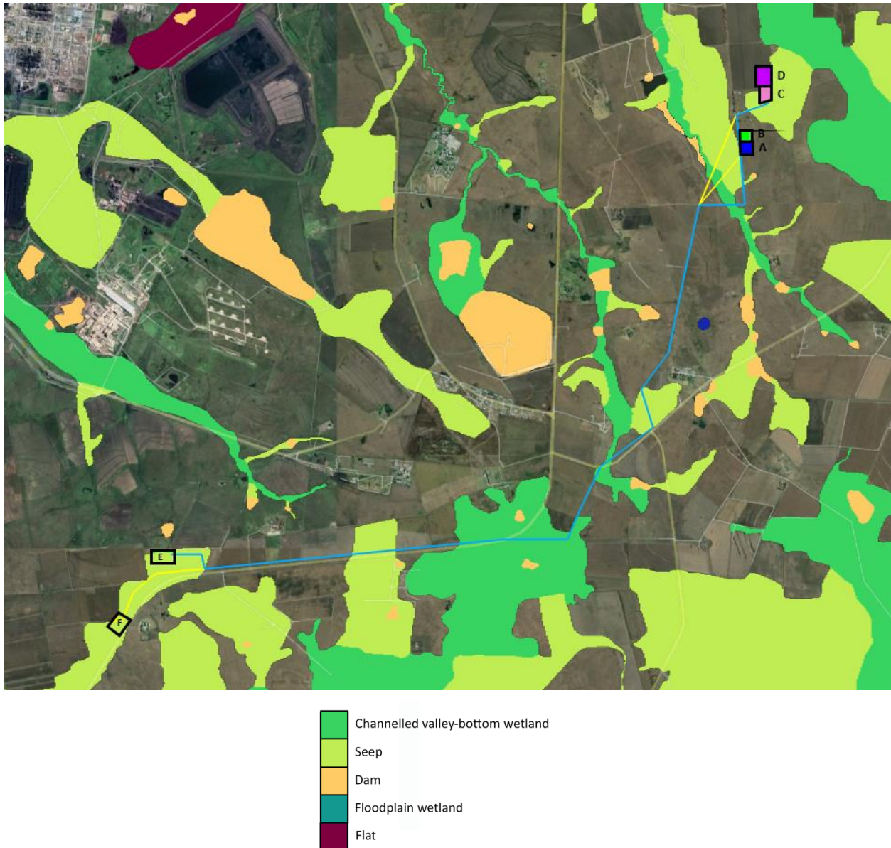
Figure 12: Mpumalanga Highveld Wetlands in the Vhuvhili gridline site (M BSP 2014; biodiversityadvisor.sanbi.org). A-B = On-site substation hub Start Alt 1 & 2; C-D = On-site substation hub Start Alt 3 & 4; E = Switching station End Alt 1 & 3; F = Switching station End Alt 2 & 4; Blue line = Alt 1 & 3; Yellow line = Alt 2 & 4.
