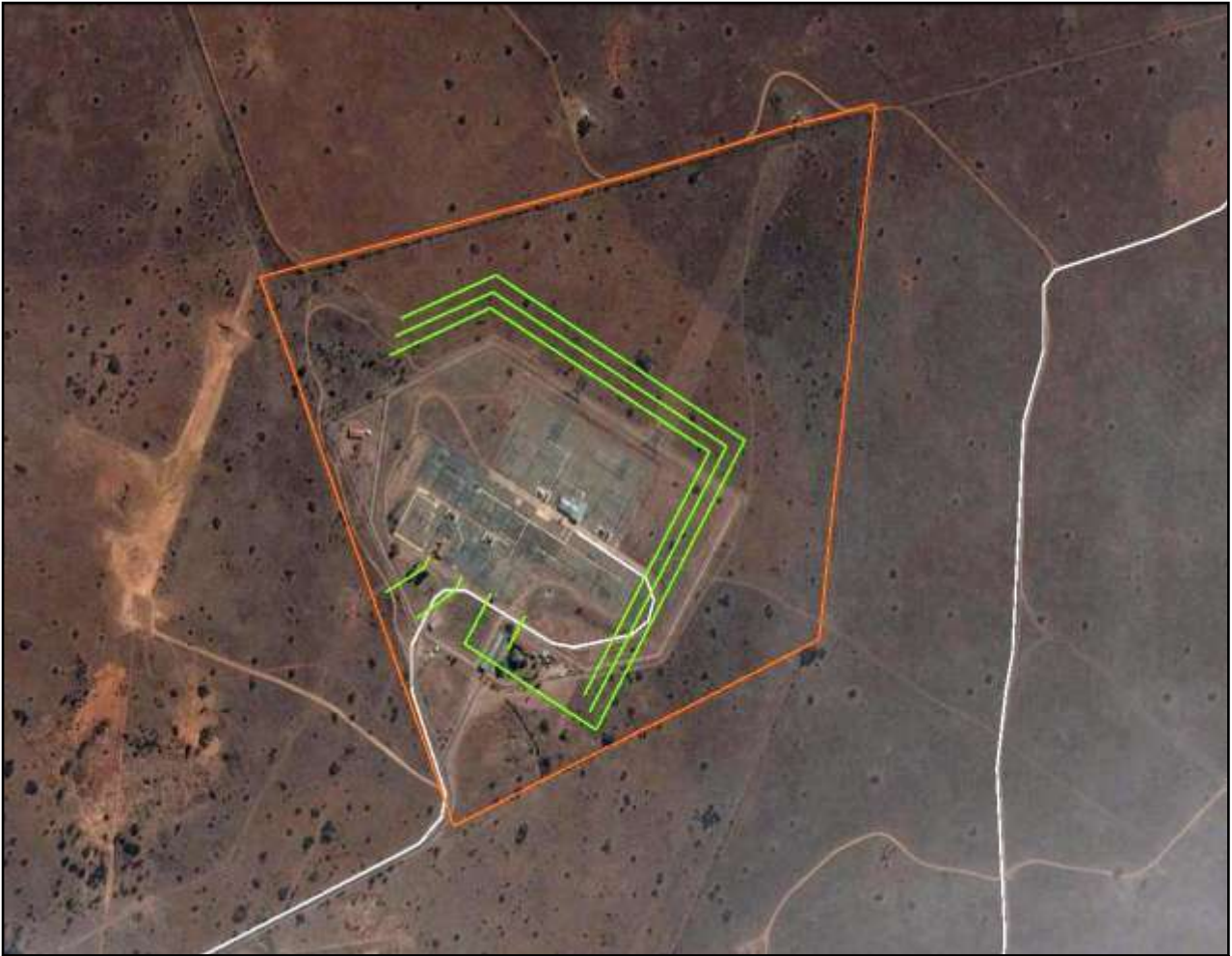
Figure 2: Proposed rerouting/relocation of 132kV lines (green).
