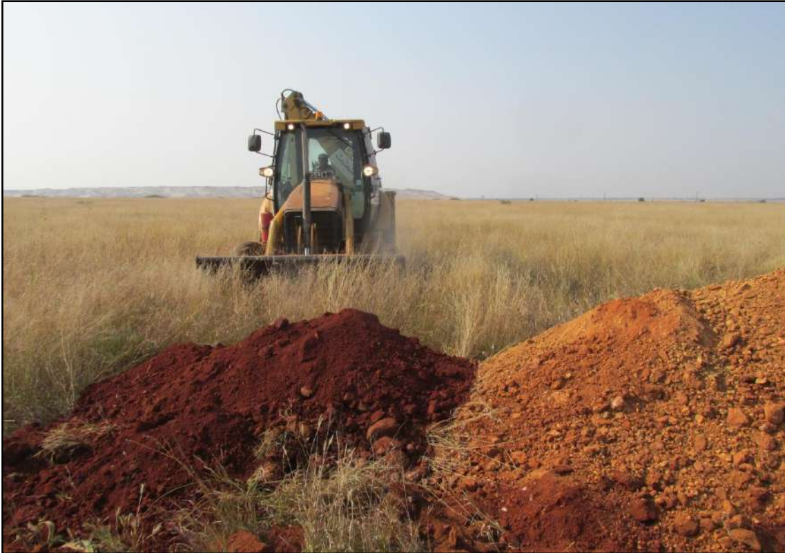
Plate 5: Upper finer reddish brown and lower yellowish brown residual andesite at TP8
