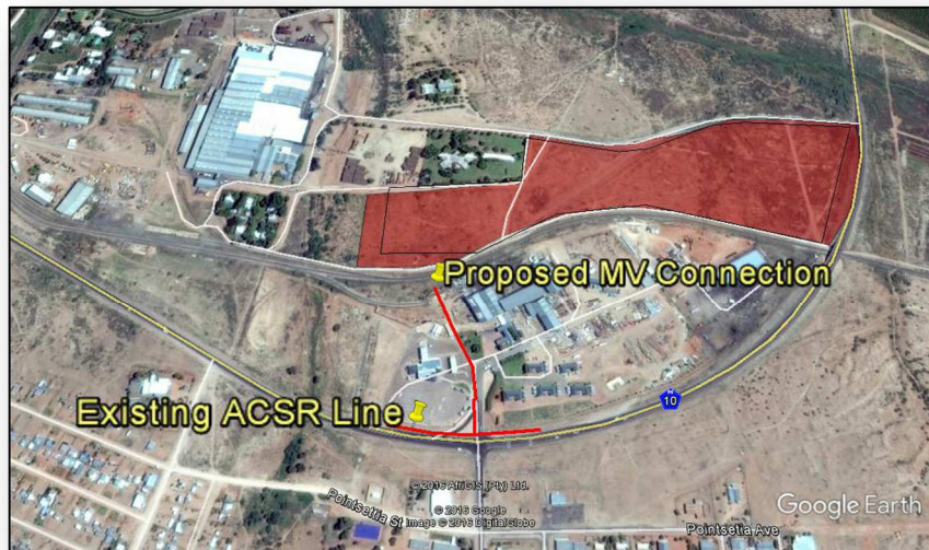
Figure 16 : Proposed Bulk Electrical Connection Point
