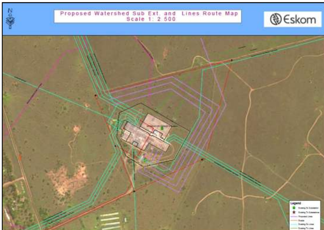
Figure 4 – Location of the proposed four additional power lines (pink lines) (from Eskom)
