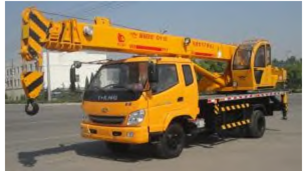
Picture 7 - 7 Tonnes Crane
