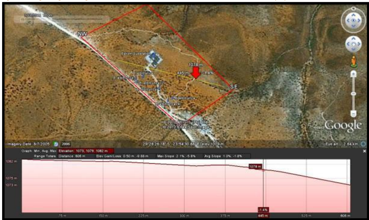
Figure 5: Google image showing the difference in elevation from the NE towards the SW corner of the proposed location
