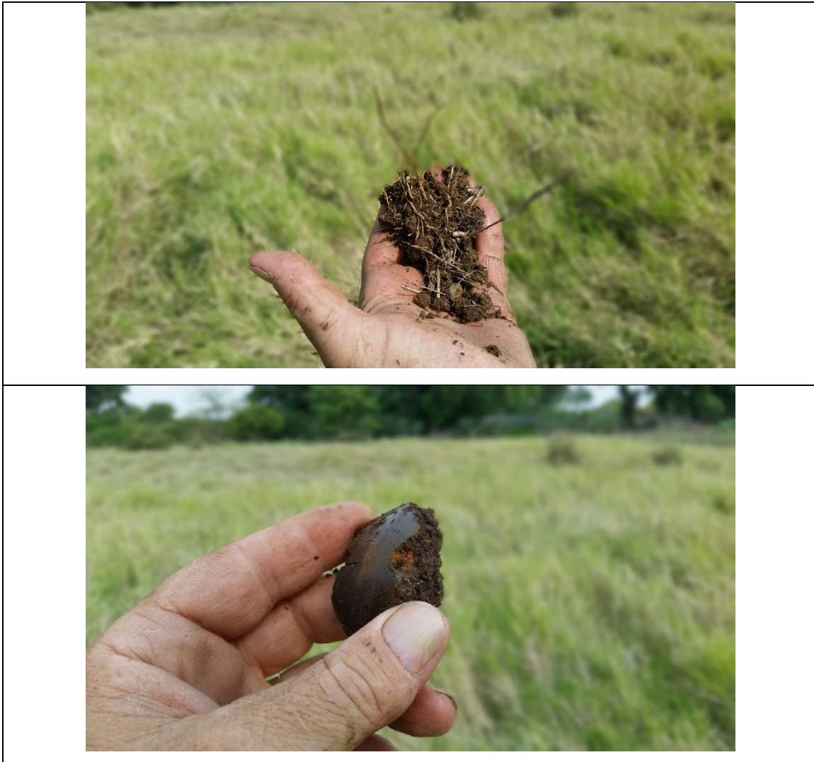
Figure 6: Illustrates selected soil features (hydromorphic indicators) recorded in the seep wetland. These include: signs of organic enrichment in the A horizon (left) and orange mottles in a dark grey matrix the topsoil profile (right).
