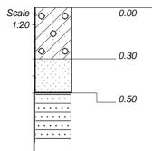
Slightly moist, orange brown,  $\underline{\text{firm}}$ , intact, gravelly sandy CLAY. **COLLUVIUM**.
