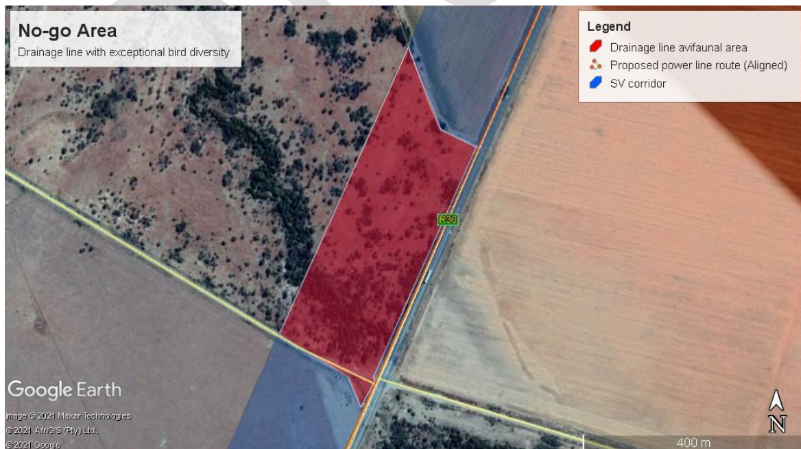
Figure 13. Drainage line avifaunal no-go area where no pylons should be placed in the drainage line and the power line should hug the R30 tarred road on the eastern side of the proposed power line corridor
