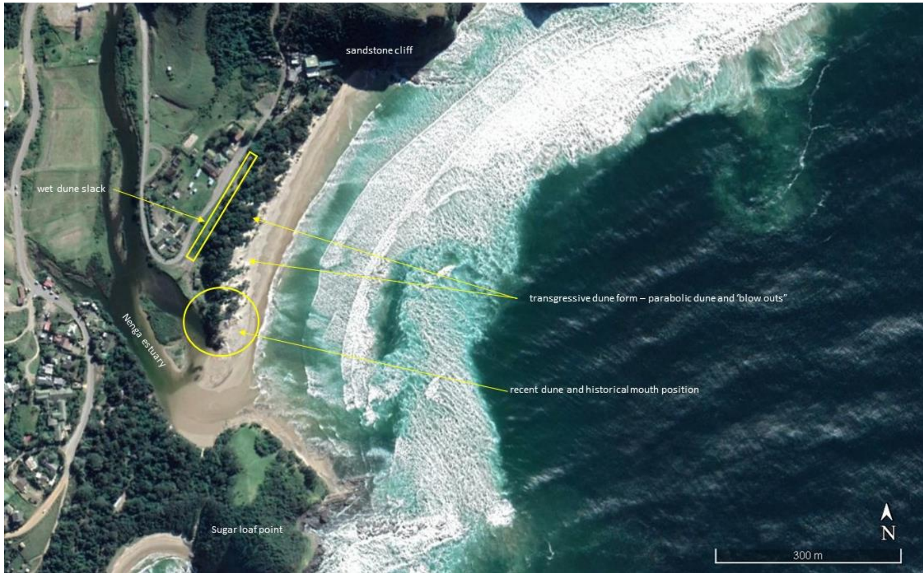
Figure 16. Aerial image of the Coffee Bay Main Beach site identifying key features along the subject coastline.
