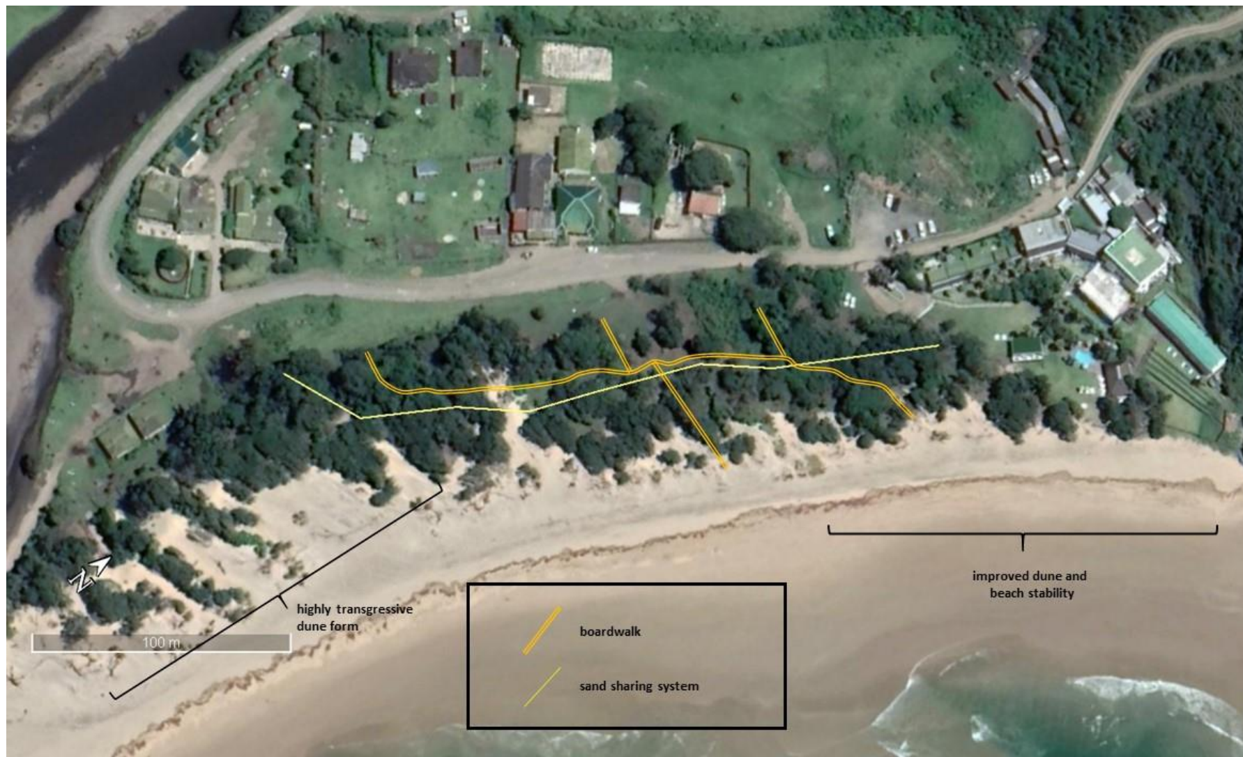
Figure 21. Aerial image of Coffee Bay Main Beach showing recommended arrangement of boardwalk in relation to sand sharing system (February 2021).
