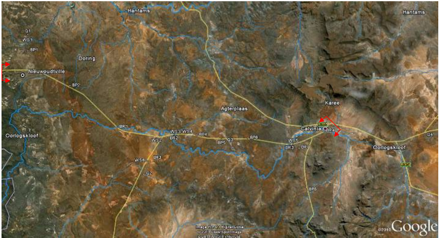
Figure 3. Aerial image of the proposed road upgrade with locality of quarries (Q), borrow pits (BP), bridges (BR) and water sources (WS)
