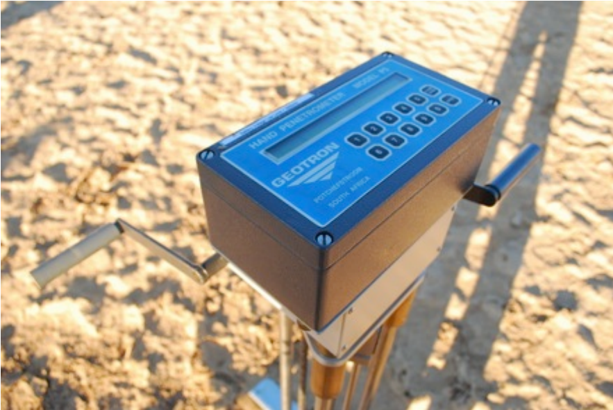
Figure 25 Hand penetrometer Model P5
