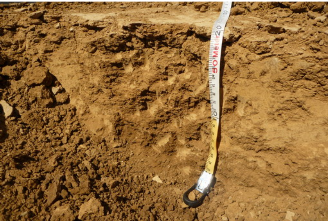
Figure 17 Exposed soil profile (20 cm) of hard pan soil without a puffy salt crust
