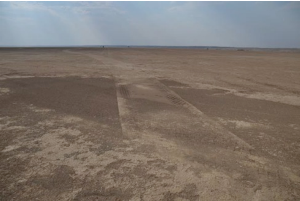
Figure 42 Bearing capacity variation and consolidation under distributed loads (wide rubber tyres) on in-filled and graded sections on Hakskeepan
