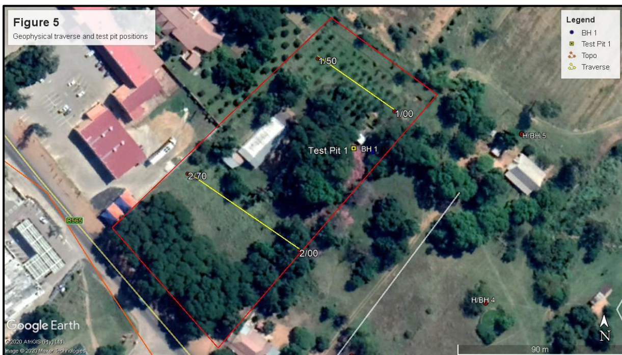
Figure 5: Position of the Test pit 1 relative to the borehole and two geophysical traverses
