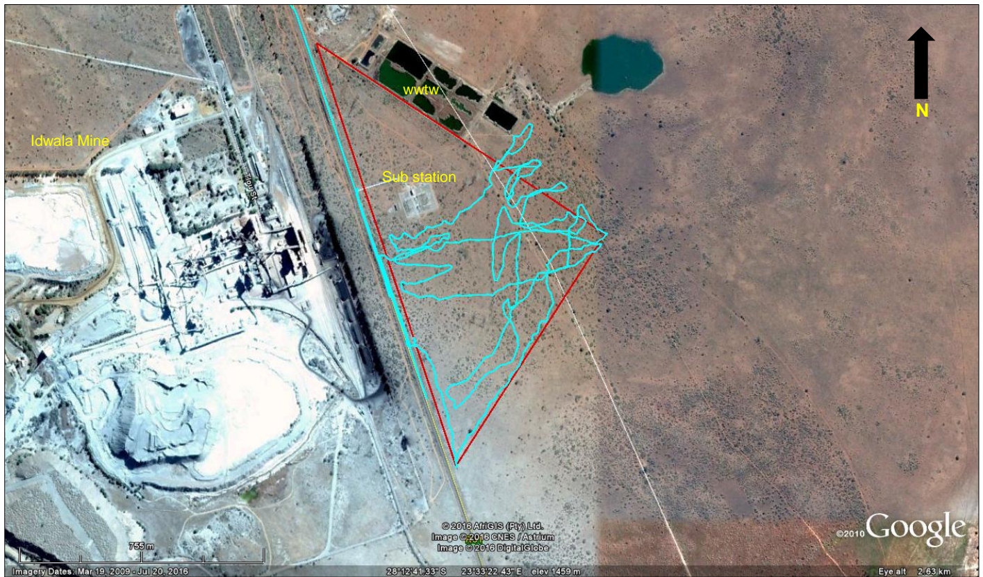
Figure 10. Track path in blue. The red polygon is the proposed 20ha footprint area, of which only an estimated 10ha will be utilized for the PV facility.
