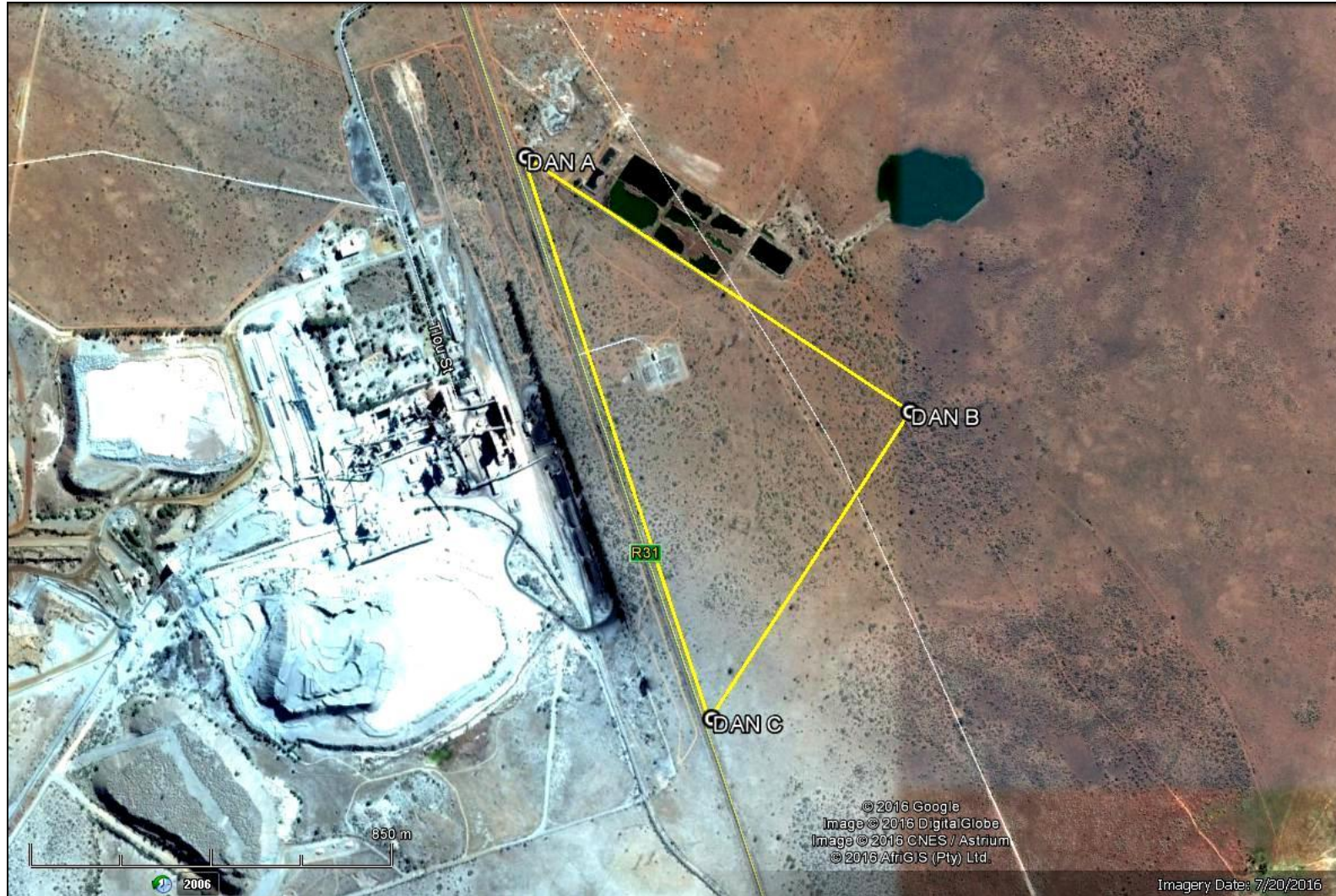
Fig. 2. Google earth© satellite image showing the flat-lying study area for the Daniëlskuil Roma Solar Plant on the south-eastern outskirts of Daniëlskuil, Northern Cape (yellow polygon). The area is mantled with wind-blown Kalahari sands with very limited bedrock exposure. The Idwala limestone mine is situated just to the west.
