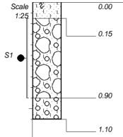
Slightly moist greyish brown loose to medium dense intact silty fine grained SAND with grass roots. Colluvium.
