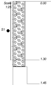
Slightly moist to dry orangey to reddish brown mottled white loose becoming medium dense to dense with depth intact silty sandy fine to coarse GRAVEL with grass roots. Residual Calcrete.
