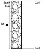
Slightly moist orangey to dark reddish brown loose becoming dense to very dense intact silty sandy fine to coarse GRAVEL with boulders and roots. Residual Dolomite. Gravel consists of fine to coarse (5-50mm diameter) subrounded dolomite fragments.
