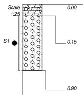
Dry light greyish brown loose intact silty gravelly fine to medium grained SAND with roots. Colluvium. Gravel consists of fine to medium (5-20mm diameter) subrounded matrix supported dolomite fragments.
