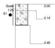
Dry light greyish brown loose intact silty fine to medium grained SAND with roots. Colluvium.
