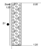
Slightly moist dark orangey to reddish brown loose becoming very dense with depth intact silty sandy fine to coarse GRAVEL with grass roots. Residual Dolomite. Gravel consists of fine to coarse (2-60mm diameter) subrounded to rounded dolomite fragments.
