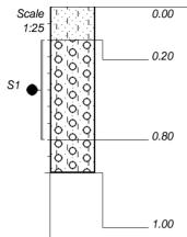
Slightly moist greyish brown loose intact silty fine grained SAND. Colluvium.
