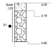
Dry greyish brown loose intact silty fine grained SAND with roots. Colluvium.
