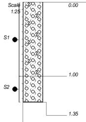
Dry dark orangey brown loose intact silty fine to medium grained SAND with abundant gravel and some grass roots. Residual Dolomite. Gravel consists of fine to medium subangular to subrounded (5-20mm diameter) dolomite fragments.
