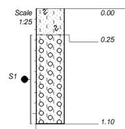
Slightly moist greyish brown loose intact silty fine grained SAND with grass roots. Colluvium.
