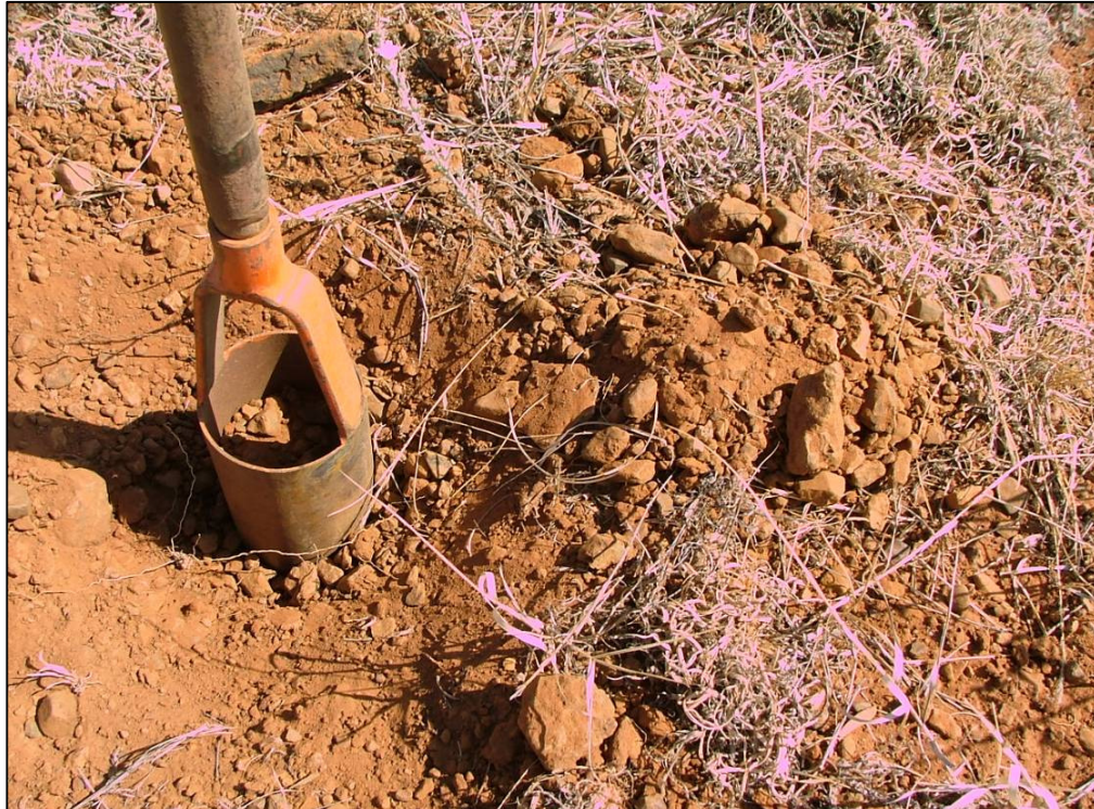
Figure 3: Soil auger indication the shallow rocky nature of the Mispah soils in the study area.
