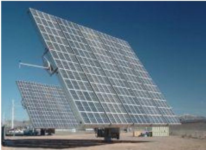
Figure 4: Typical CPV Unit
