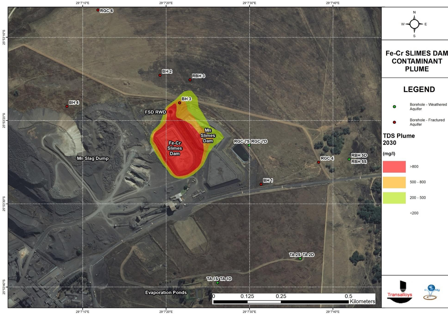
Figure 4.5: Impact from the Fe-Cr slimes dam (8 years after rehabilitation)
