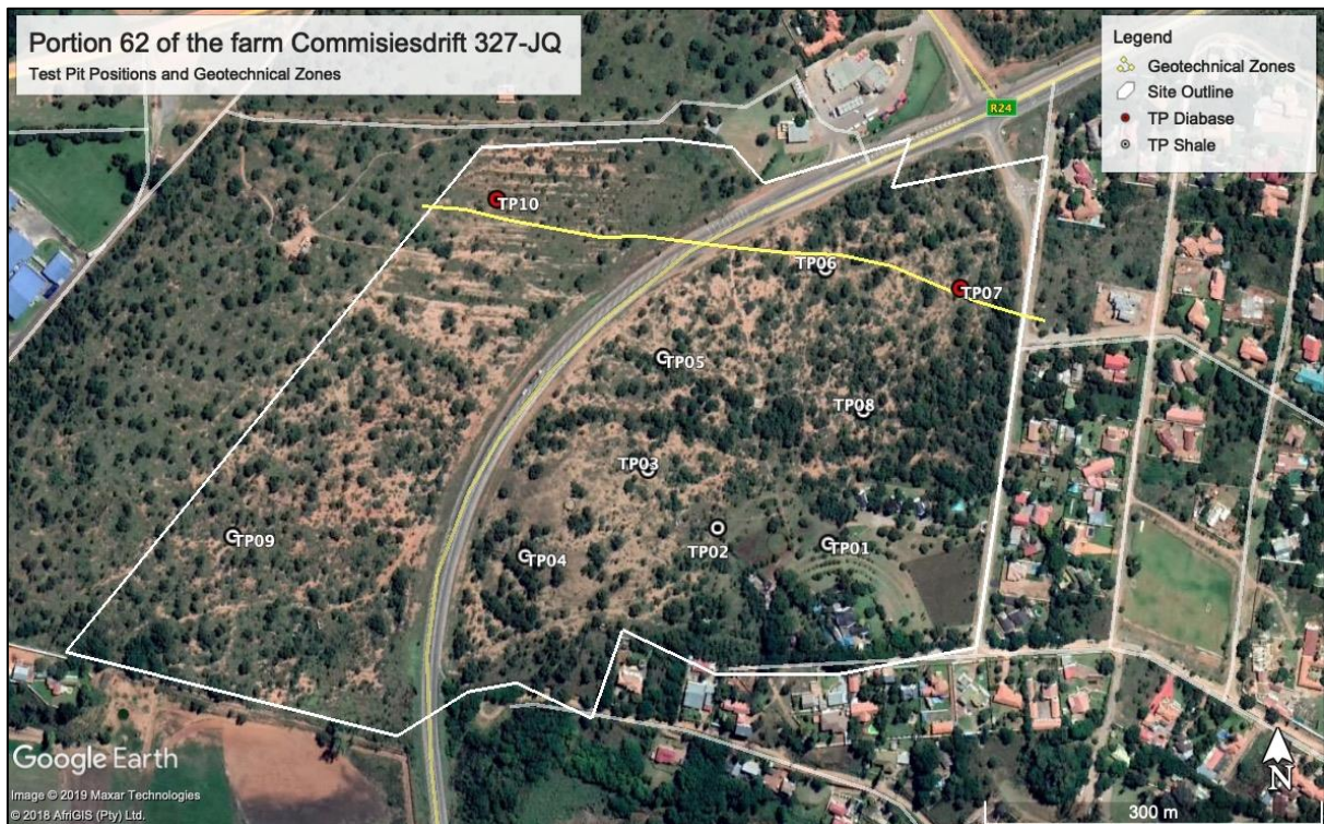
Figure 4: Test Pit Positions
