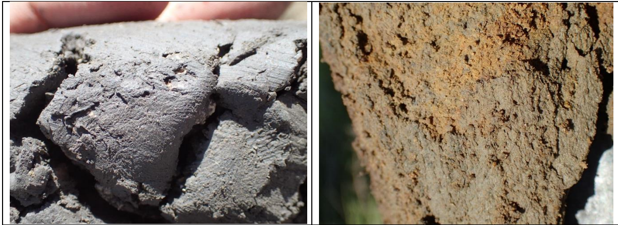
Figure 4: Illustrates wetland indicators in the form of gleying with distinct grey colours recorded in a soil sample with a high clay content from near the centre of a valley bottom wetland (left); and a sample from the outer portion of a valley bottom wetland with orange mottling and surrounding light grey areas caused by iron depletion due to a fluctuation in soil saturation typical of a temporary wetness zone (right).
