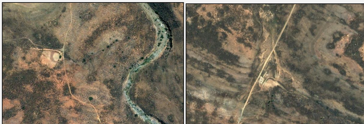
Figure 14: Digital satellite images depicting small instream impoundments located within episodic drainage lines.
