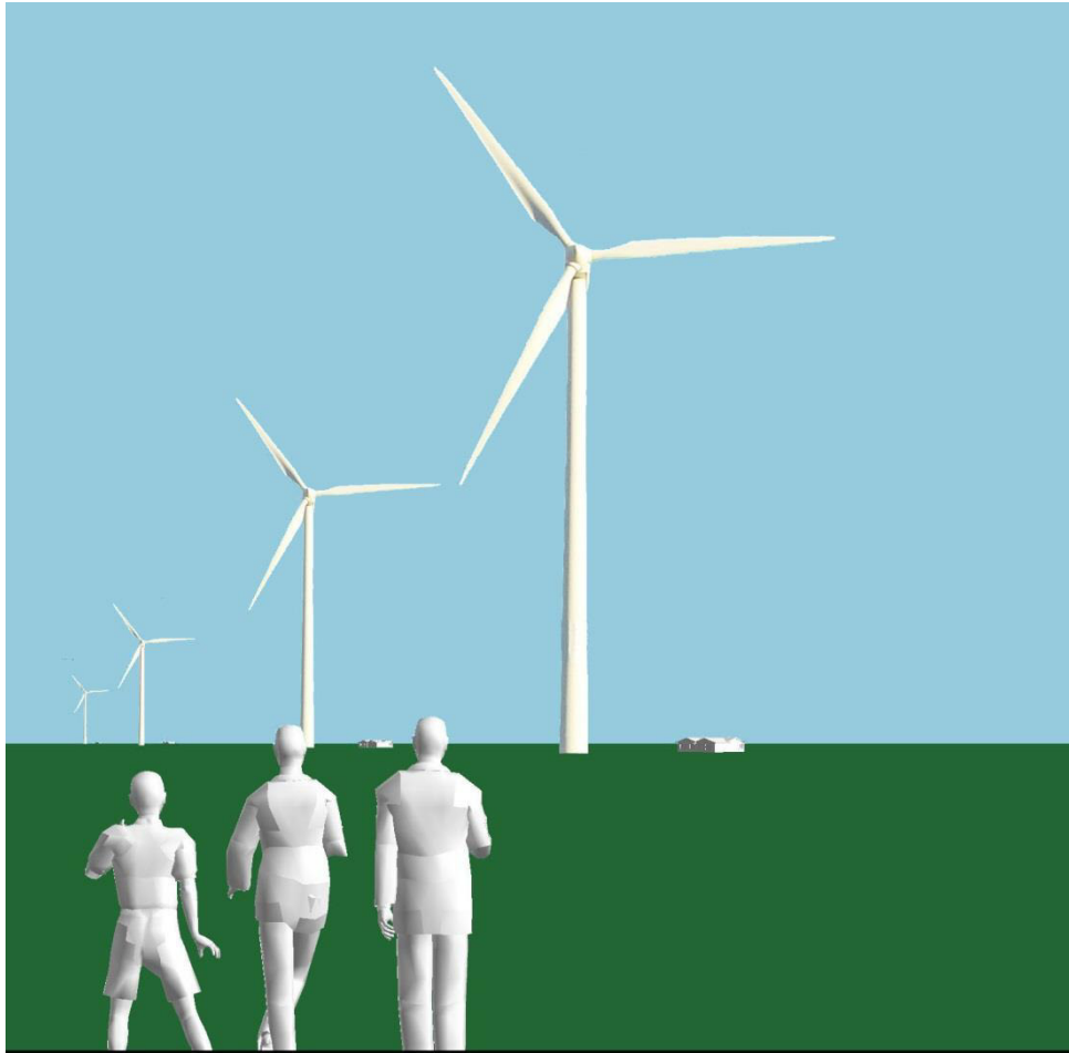
Figure 6: Schematic representation of a wind turbine from 1, 2, 5 and 10km under perfect viewing conditions.
