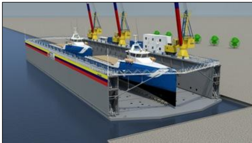
Figure 3. Vessels moored in a floating dry dock awaiting repairs (image courtesy of Nestoil).
