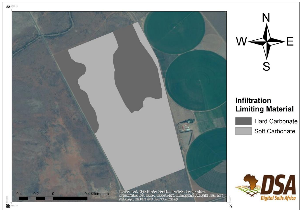
Figure 8: Water infiltration limiting material distribution.
