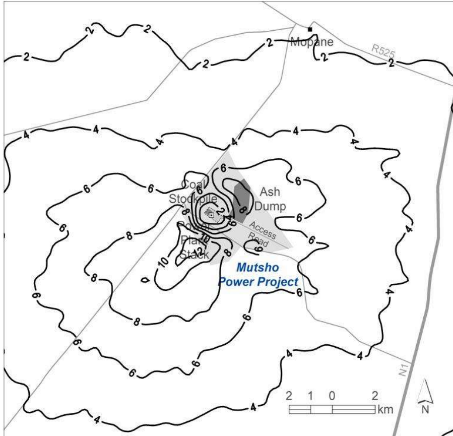
Figure 15: Predicted 24-hour average SO 2 ambient concentrations in µg/m 3 resulting from emissions from the proposed Mutsho Power Project Boiler Stack in Isolation for the preferred site layout
