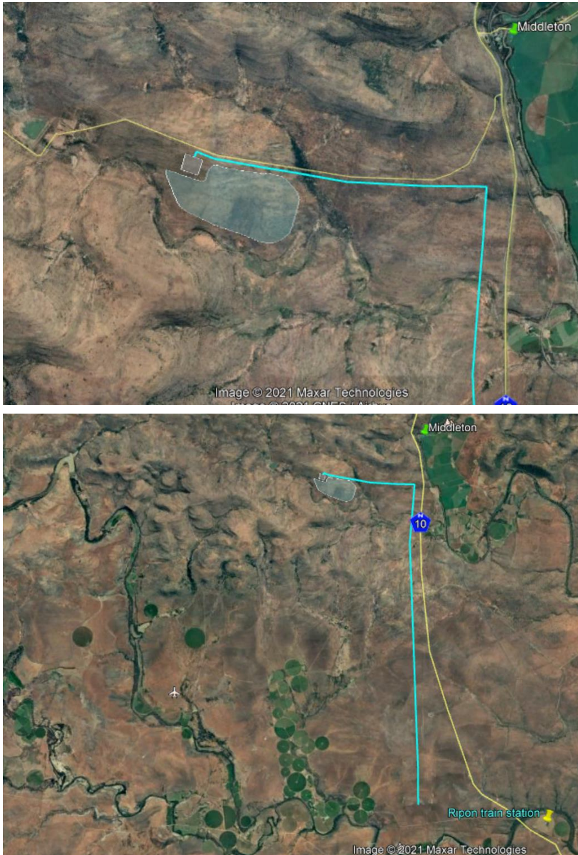
Figure 3a. GoogleEarth images showing Ripponn BoP area shaded light green, 132kV collector sub (above) and the light blue line (below) is the 16km powerline connecting to the proposed 400kV sub where it will connect the existing Eskom 400kV powerline.
