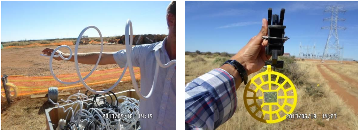
Figure 27: Examples of bird flight diverters to be used on the power lines: Double loop bird flight diverter (left) and Viper live bird flapper (right).
