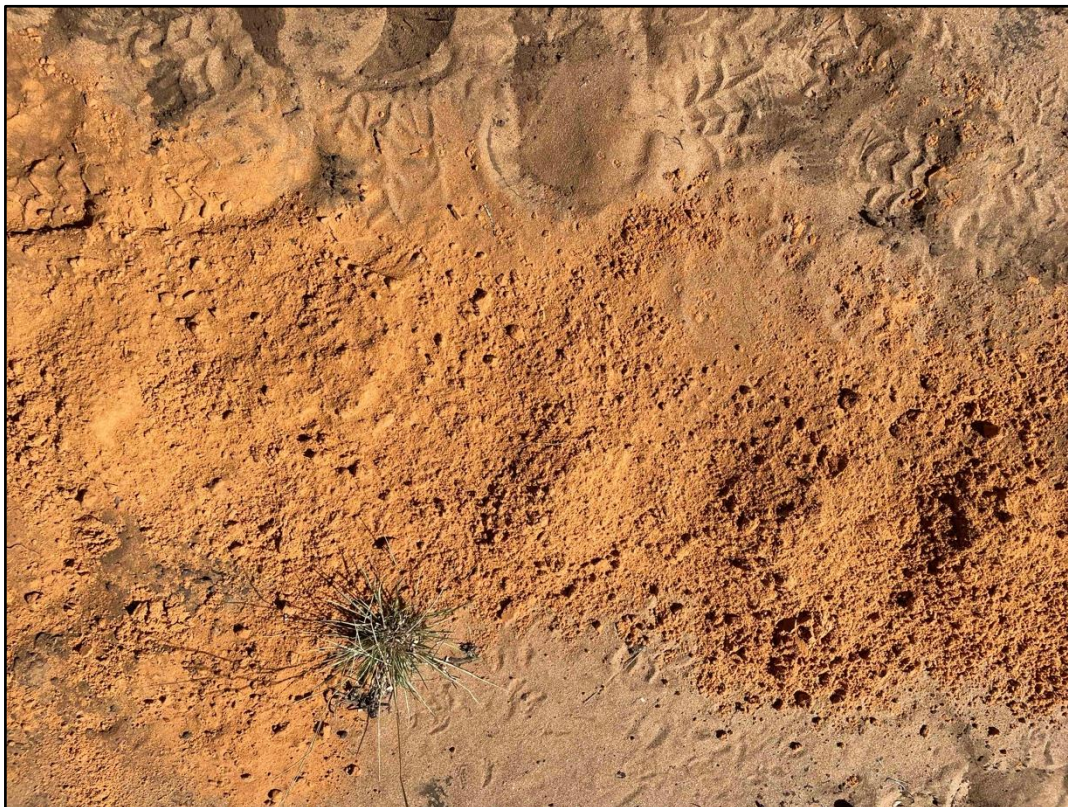
Figure 8 Example of the yellow colour of the apedal subsoil (in the middle) that was placed on the surface where the bleached colours of the topsoil can be seen (bottom and top of photo)
