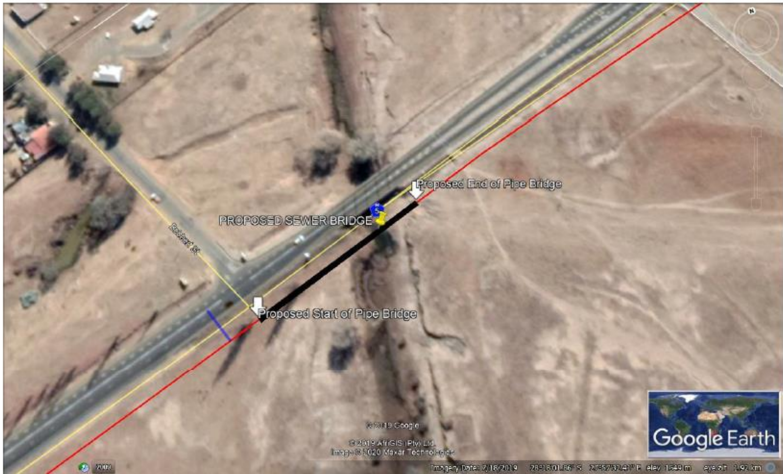
FIGURE 1: MAP DEPICTING PROPOSED SEWER PIPE BRIDGE
