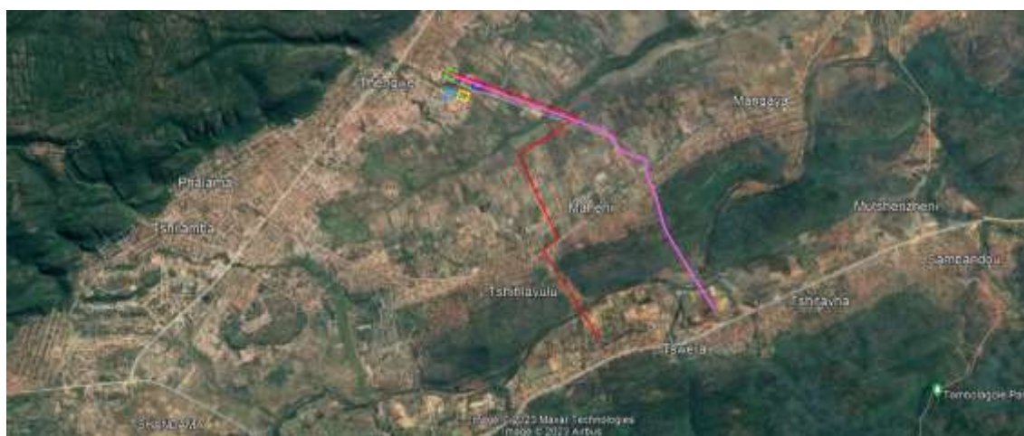
Figure 1.1: The aerial view of the proposed project – the purple line represent Alternative 1 and the red line Alternative 2 of the power line corridors, with the coloured blocks the proposed substation sites (four alternative substation sites).
