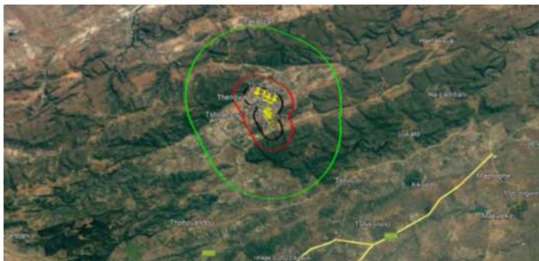
Figure 3.36: A general view of the proposed corridor for power line (Alternative 2) with the KOPs and the visual exposure rating distances (as described in Table 1 – black circle = 1.5 km, red circle = 3 km and green circle = 10 km) indicated.
