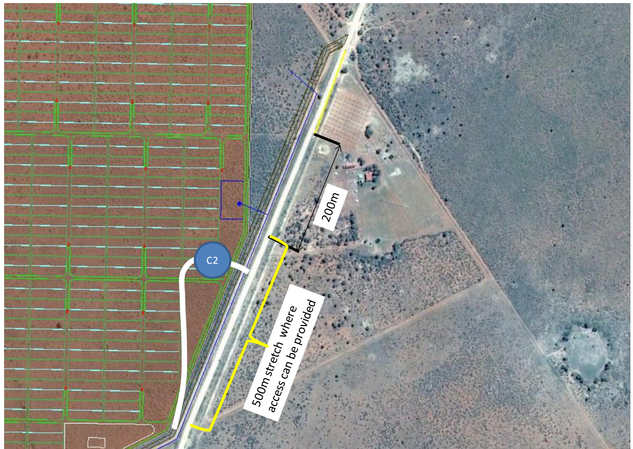
Figure 4.8 Access Spacing at the Recommended Position - Alternative 2
