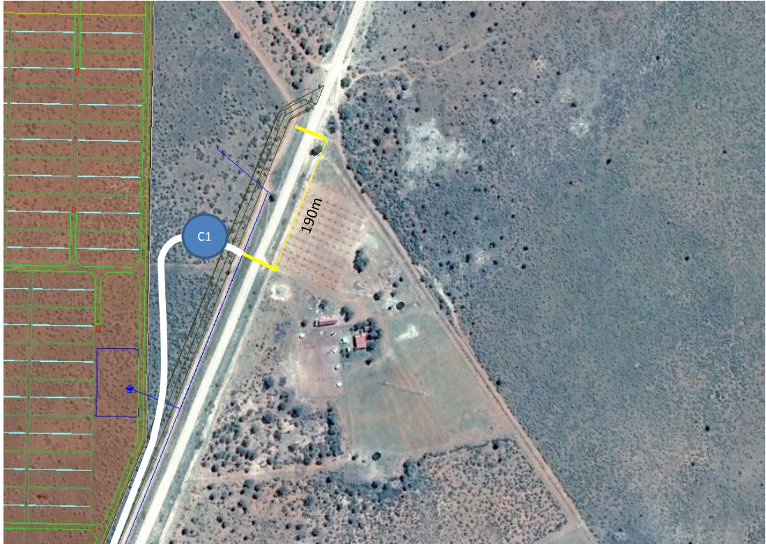
Figure 4.7 Access Spacing at the Recommended Position - Alternative 1
