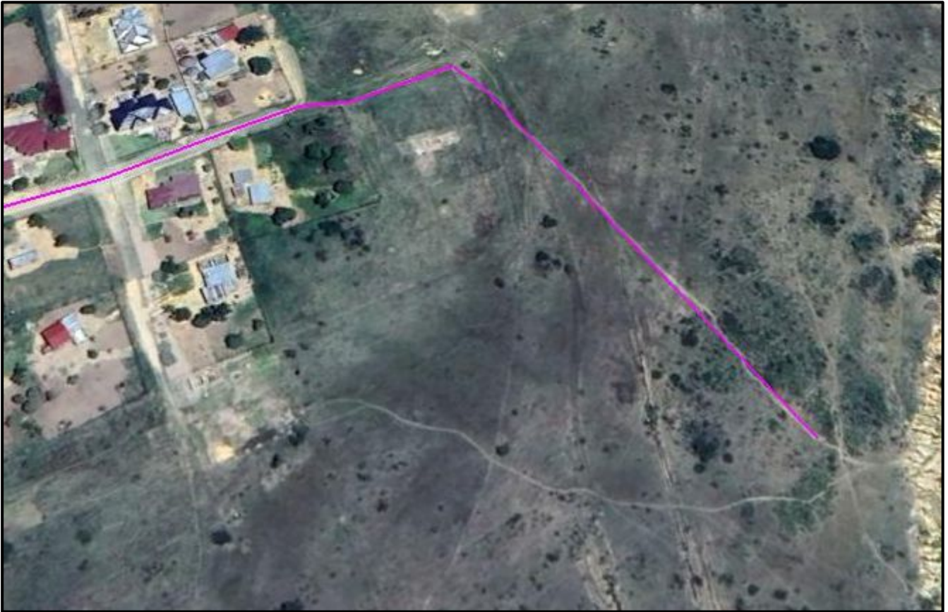
Figure 8 Proposed alternative access road required west of the dam to access the spillway channel on the right embankment.
