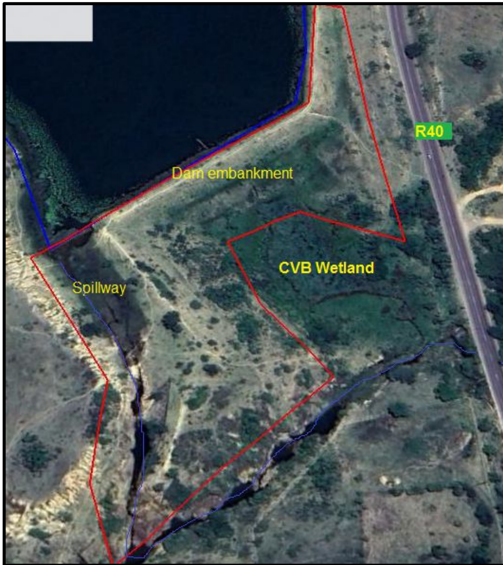
Figure 7: Rehabilitation works area superimposed on Google Earth Satellite imagery showing the site is covered in disturbed veld/open bushland, a CVB wetland and the Tlulandziteka River. The area has been disturbed in the past by the construction of the dam.
