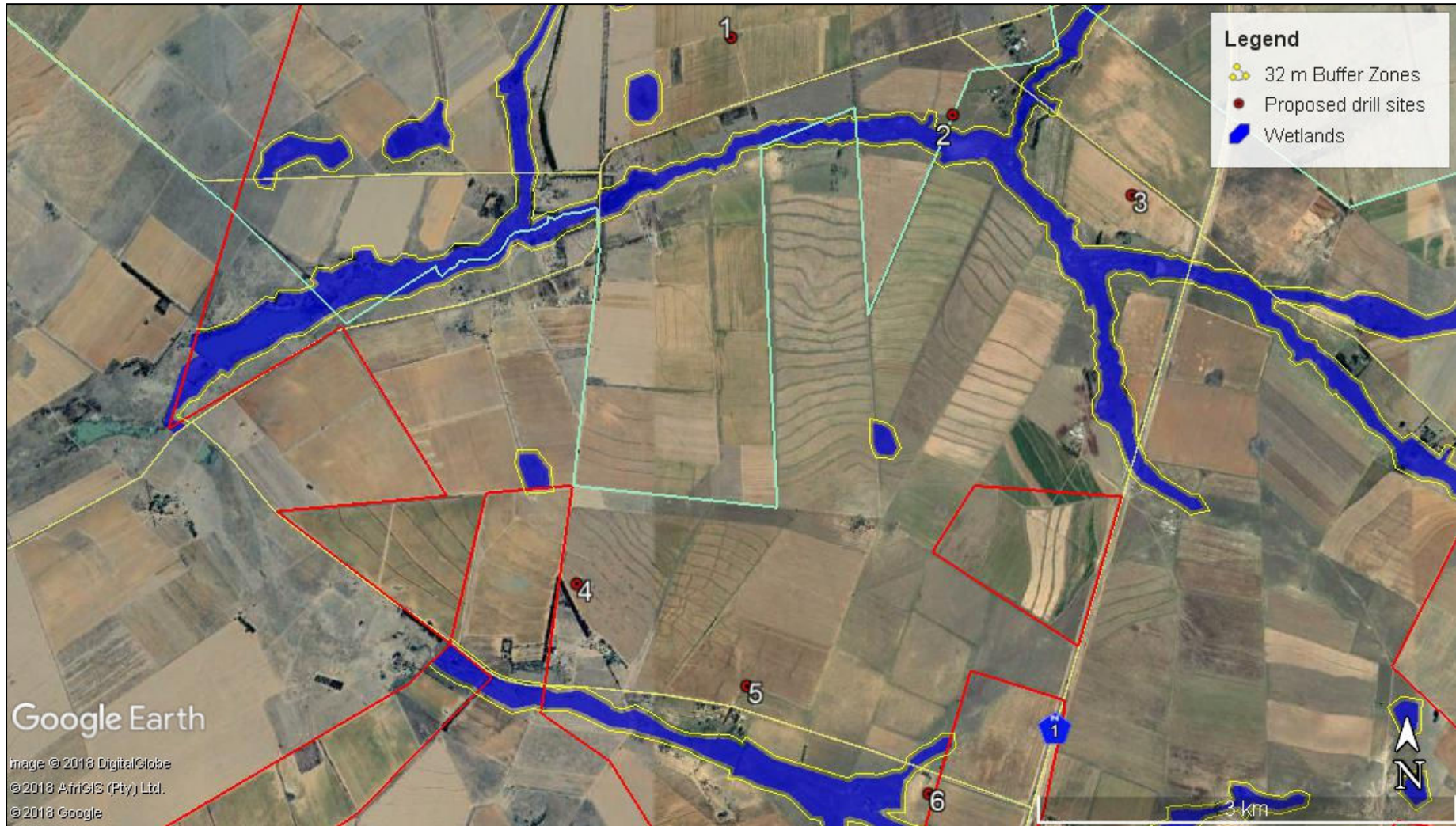
Figure 20: Delineated wetlands with 32 m buffer zones relative to the proposed positions of six drill sites.
