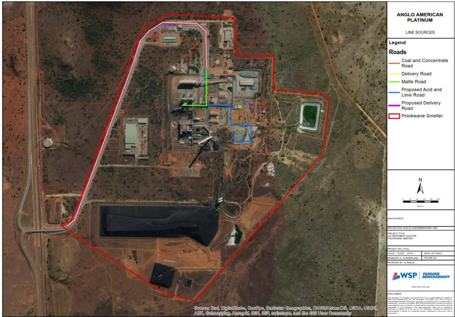
Figure 6-2: Layout of roads at Polokwane Smelter.
