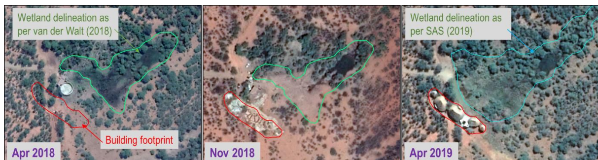
Figure 19: (Left) the proposed building footprint relative to the delineated wetland by van der Walt (2018); (center) the construction footprint and delineated wetland during the construction phase; (right) the constructed buildings relative to the anthropogenically extended wetland, delineated by SAS (2019).
