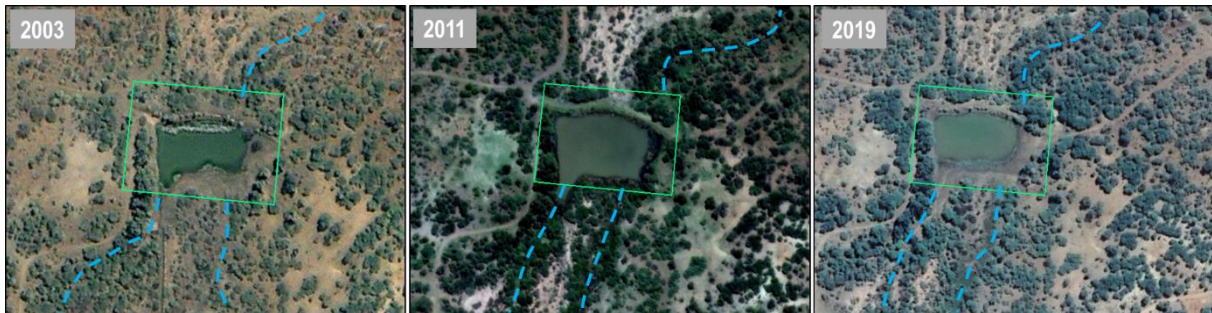
Figure 23: Digital satellite imagery of Dam 2 within an ephemeral drainage line (blue dashed line), in 2003 (left), 2011 (center) and 2019 (right).
