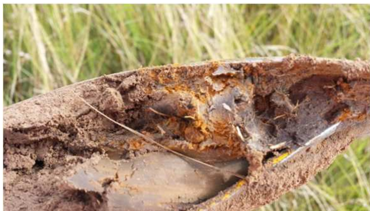
Example of a wetland soil extracted during the wetland delineation, with typical grey soil matrix and extensive orange mottling characteristic of a 'seasonal' zone of saturation.
